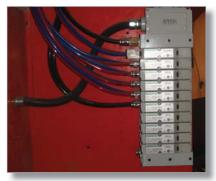
Pneumatic valve controls for Archer Batching System
